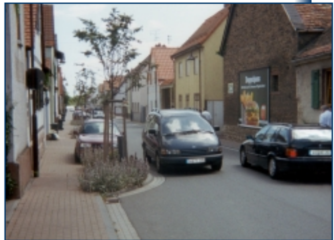
Figure 16. Landscaping to narrow lane width, Germany.
